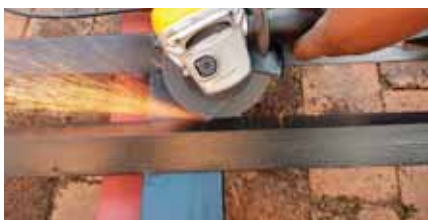
Grind the original gate
