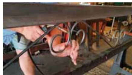
Weld scrolls in place
