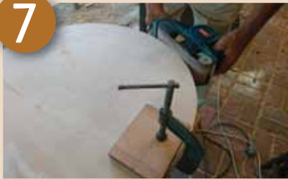
Use a 'blokkie' to protect the surface!
