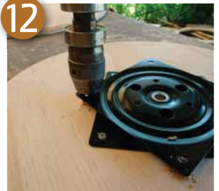
Attach the swivel plate
