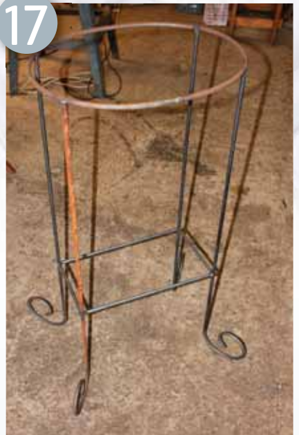
Grind all joints
