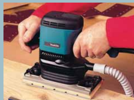
Most sanders come equipped with a dust collection bag or can be connected to a vacuum cleaner
