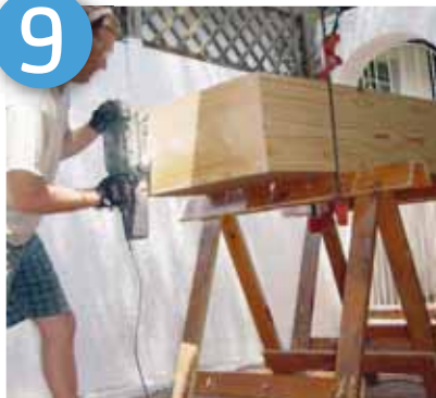
Sand off any protrusions from the joints
