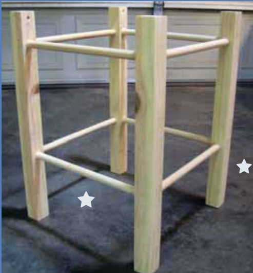
The four legs held together with the aid of the dowels
