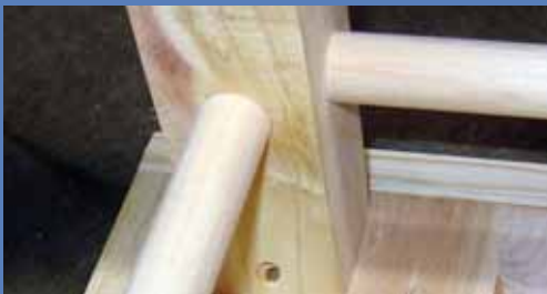
Close-up of the legs showing how the dowels fit neatly into the round recesses
