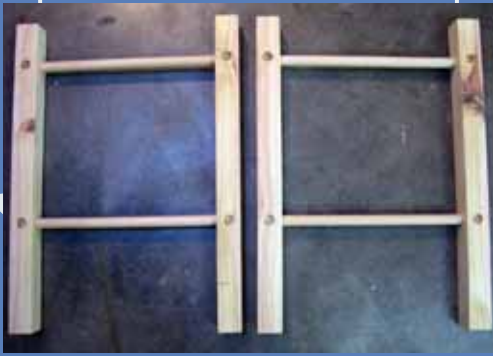
The assembly of the legs showing the dowel placement
