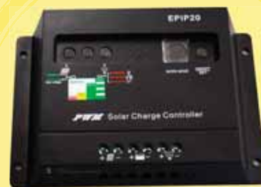
The solar charge controller receives and manages power coming from the PV panels
